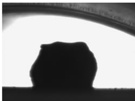
Fig. 10: Slag on \text{Al}_2\text{O}_3 at approx. 1365°C
