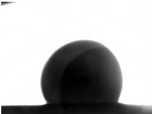
Fig. 5: Slag sample on graphite at approx. 1635°C
