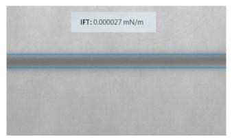
Fig. 3: Exemplary image of a drop of a microemulsion in the surrounding heavy aqueous phase for the system water-NaCl-*n*-heptane-AOT. The rotational speed was set to 1400 rpm. The drop was fitted according to Vonnegut.
