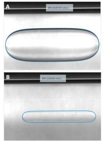
Fig. 1: Exemplary drop images of sample 1 (A) and sample 7 (B). The rotational speeds are 12000 and 6000 rpm, respectively. Drops were fitted according to Young-Laplace.
