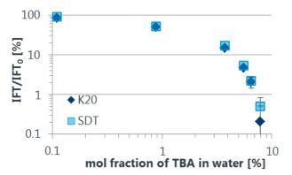
Fig. 2: Plot of normalized IFT (IFT divided by IFT of water vs. CHX without TBA =  $IFT_0$ ) vs. molar fraction of TBA in water at equilibrium conditions. The data for spinning drop (light blue) and K20 (dark blue, [1]) overlap very well, while the standard deviation (error bars), especially for low IFT, is much smaller for SDT compared to K20.
