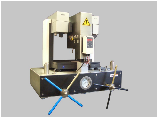
Fig. 5: Measuring apparatus PA3210 for measuring the interfacial tensions and contact angle under pressures of up to 700 bar and temperatures up to 200°C.
