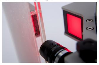
Abb. 3: View of the camera to the foam-wetted prism of the Foam Structure Module – FSM
