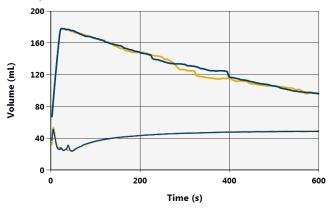
Fig. 4: Example Holsten Pilsener: the maximum foam volume and the decay (upper curves) and the change in liquid volume below the foam column (lower curves) can be reproduced very well.
