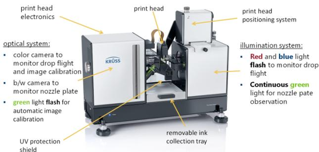
Fig. 1: Construction of the DSA Inkjet with fitted print head
