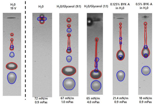
Fig. 6: Drops of different liquids each jetted with 21 V and 8 μs. The drop generation for water with a pulse height of 19 V can be seen on the far left.
