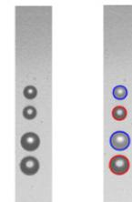
Fig. 3: Double-exposed image of a flying drop; right with contour detection. The software automatically and unambiguously associates the images with the red and blue flashes and therefore with the respective points in time, and outlines the drops in the appropriate colors.
