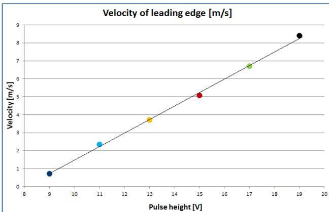
Fig. 5: Velocity of the leading edge as a function of pulse height determined with ADVANCE. The colors of the data points correspond to the outlines of the corresponding drop images in Fig. 4.
