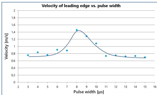
Fig. 8: Velocity of the leading edge as a function of pulse width at a pulse height of 9 V for a solution of 2% BYK-B in water
