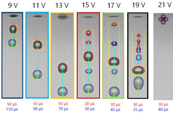
Fig. 4: Images of water drops dosed with a pulse length of 8 μs at different pulse heights
