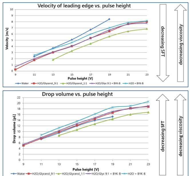
Fig. 7: Velocity of leading edge (top) and drop volume (bottom) for liquids of different SFT and viscosity at different pulse heights
