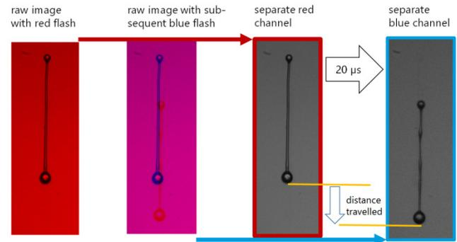
Fig. 2: Image generation in the DSA Inkjet. A red flash is produced at a specified delay time after the piezo pulse. After a further time (here 20 μs) the same image is illuminated in blue. The color channels are then separated, which enables the drop velocity, for example, to be determined.
