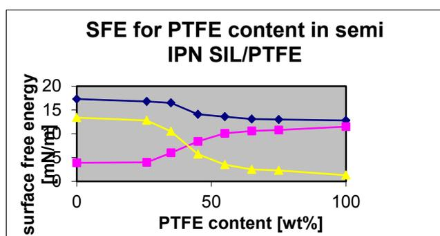
Knowing the different molecular structure of PTFE and SIL it is clear that in such aqueous coating formulations increasing PTFE/SIL ratio results in increased water contact angle and decreased SFE value. As one can see,
